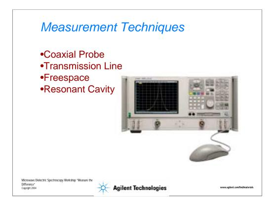
Today, we will be demonstrating techniques that use a microwave Network Analyzer. The Network Analyzer is useful because it is broadband, 300KHz to 325Ghz, and it's general purpose capabilities make it useful for a variety of techniques. The Impedance Analyzer offers additional techniques for lower frequency applications.
