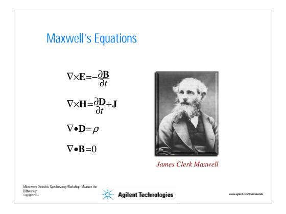
The solution of Maxwell's equations determines how microwave energy propagates through a material. Maxwell's equations can be expressed in many equivalent forms. Its most general form is listed here.
