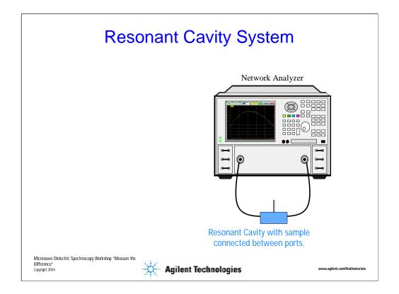
The resonant cavity system consists of a resonant cavity connected between two ports of a network analyzer with coax cables. The dielectric properties can be calculated from the transmission response of the cavity, measured empty and then with the sample. The calculation can be performed manually, or from user written software controlling the network analyzer over LAN or GPIB.
