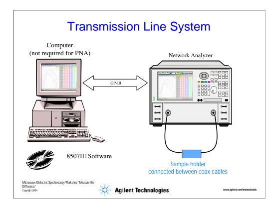
A typical transmission line system consists of a vector network analyzer and a sample holder connected between the two network analzyer ports. Agilent provides software that converts the reflection and transmission coefficients to dielectric properties. For the PNA series network analyzers, a computer is not required as the software can be run directly on the instrument. For all other network analyzers, an external computer with HP-IB card is required.
