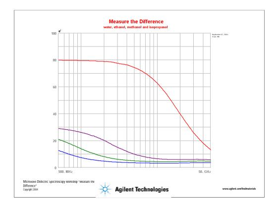
Here's a look at water and three different alcohols. The X axis of the graph is frequency and the Y axis is the real part of permittivity, which represents a materials ability to store energy. The red trace is water.
