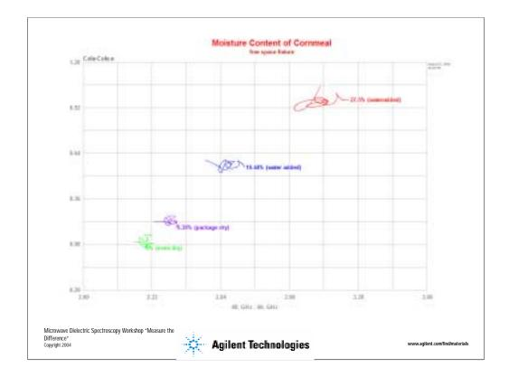
This is a measurement of Cornmeal samples with different levels of moisture content measured with a freespace system. The graph shows a Cole-Cole display. You can see that both the real part, on the x axis, and the imaginary part, on the y axis, increase as the moisture content increases. The University of Georgia has done some in depth work correlating moisture content to dielectric properties.
