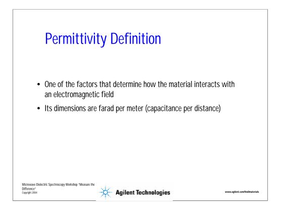
The dielectric properties, or permittivity, is one of the factors that determines how a material interacts with an applied electromagnetic field.
