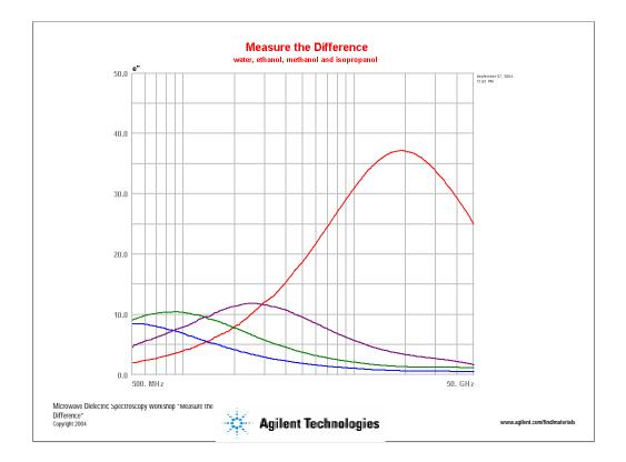
Here we are looking at the same measurement as the last slide, but the x axis is now the imaginary part of permittivity. So, we are looking at the lossiness of our material. You can see that each alcohol and the water have their peak loss at different frequencies.
