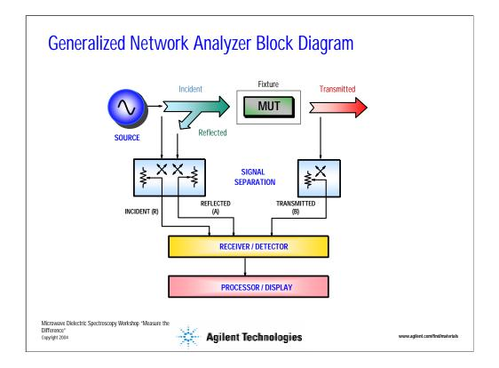
Here is a generalized block diagram of a network analyzer, showing the major signal-processing sections. In order to measure the incident, reflected and transmitted signal, four sections are required:
