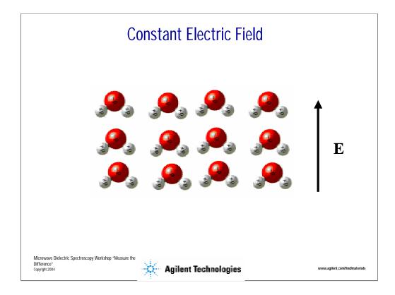
If a constant electric field is applied to this group of water molecules they will tend to orient with the applied field. This orientation ,or polarization, causes the water to have a particular capacitance per meter.
