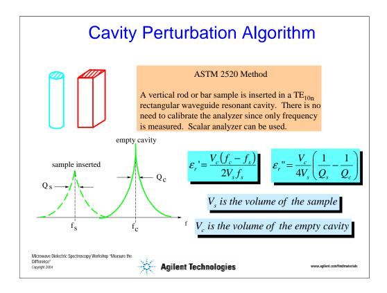
The ASTM 2520 is a fairly simple and commonly use method. This algorithm is dependent on the center frequency and Q measure with and without the sample inserted. The volume of the empty cavity and sample are also required. Other more accurate and complex methods have been developed at NIST.
