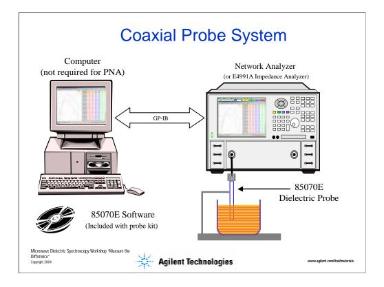
A typical coaxial probe system consists of a vector network analyzer, a coaxial probe, an external computer with HP-IB card and software. For the PNA series network analyzers, a computer is not required because the software can be run directly on the instrument.
